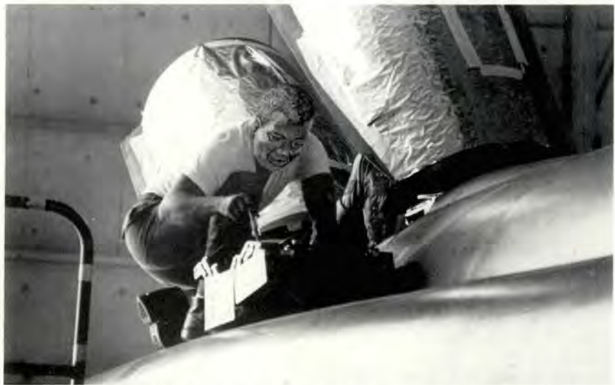
Strict control of tools and hardware is an absolute must when working in or around the phantom's vari-ramps. Loose hardware in the vari-ramp area is a major source of engine FOD.
